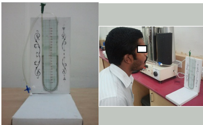
[Table/Fig-1]: Mercury manometer used in this study. Green colored head end of Ryle's tube, Ryle's tube filled with mercury column in a U-shape, graduated graph sheet and 3- way connector to be used at mouth piece end are shown.
